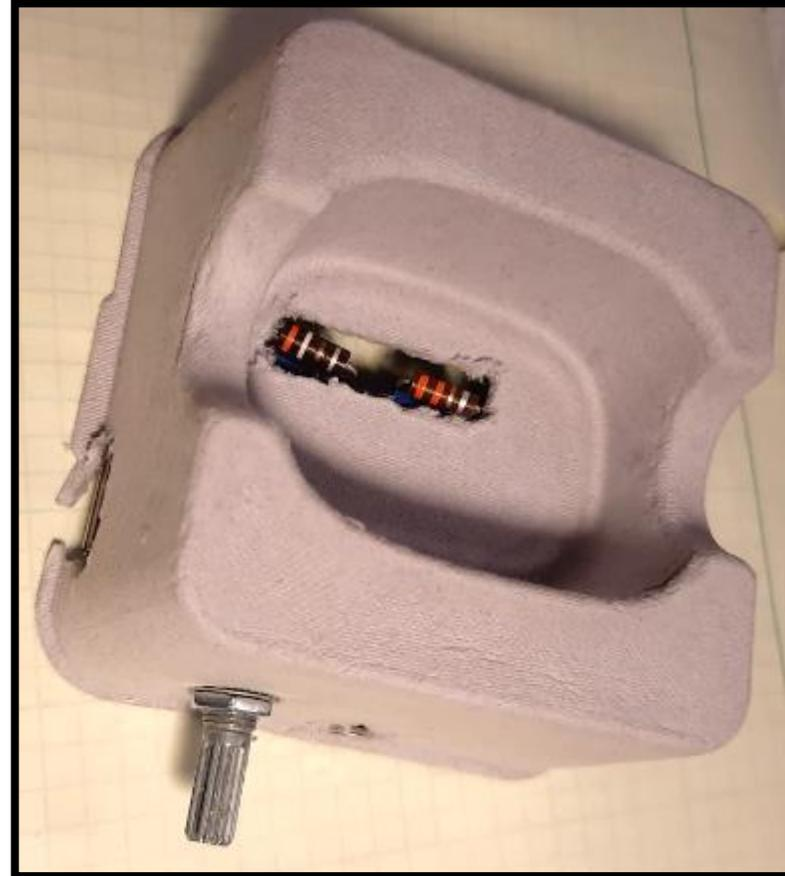
The cardboard shell is placed back into the box along with the Aeotec sensor. The mounting hardware for the volume control hold the amplifier in place with the knob pushed onto the volume control's shaft.
