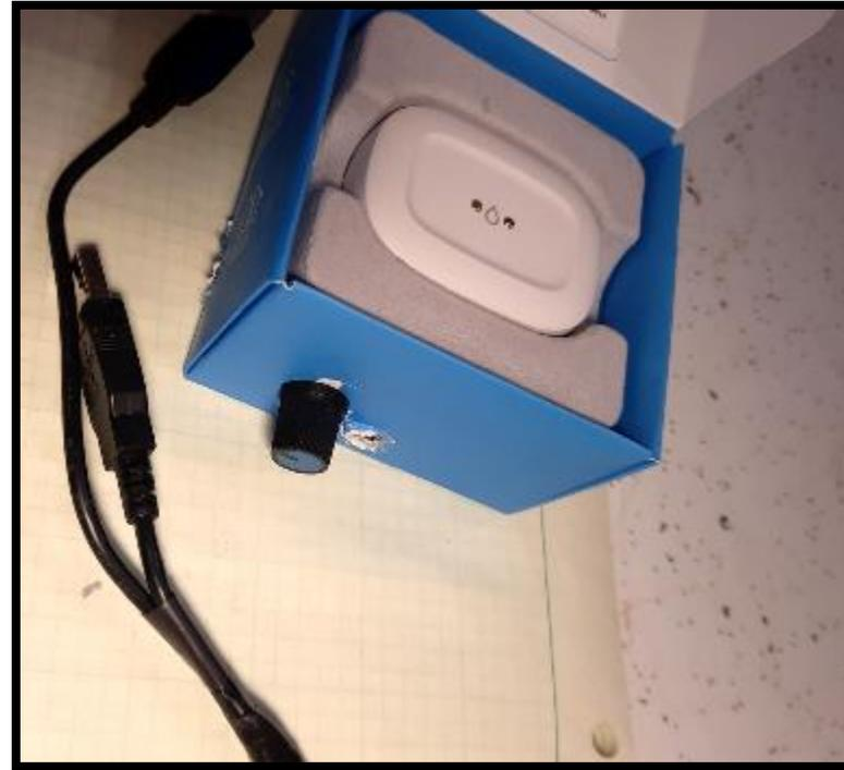
I placed the Dead Air monitor in a place where its temperature would be less affected by external heat sources such as the PC and baseboard heaters. I set the volume knob to about 2 o'clock to start and ended up leaving it there. The typical voltage across the  $3.3\Omega$  resistor peaks to around 0.5V which works out to just over 0.076W - well under the 0.25W rating.
