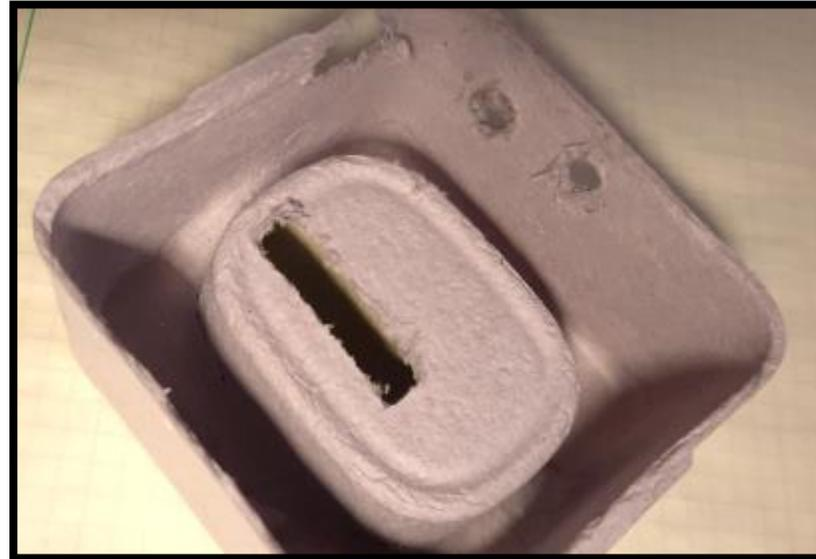
Here is the amplifier installed into the cardboard shell that holds the Aeotec temperature / leak sensor. The open hole for the resistors allows heat to reach the sensor more quickly.
